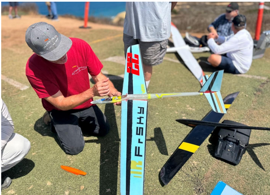
Mike Frandsen reviewing his very nice Vortex for the modelers at Torrey which makes use of foam, fiberglass, and printed products in specific locations. Very neat! Will be in production soon. (Bob Hirsch photo)
